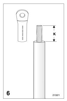
Cut back the insulation according .o dimension **K** = depth of cable lugbarrel hole + 5 mm.
