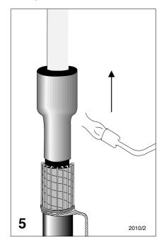
Place the stress control tubing (black) over the core and position it so that it is level with the oversheath cut.
